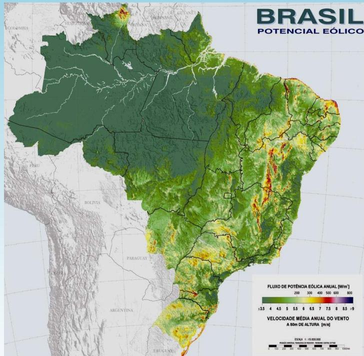
The Wind Atlas of Brazil (2001) presents an estimated potential of **143 GW**, using a reference height of **50 m**, and the state of the art equipment of 600kW.
